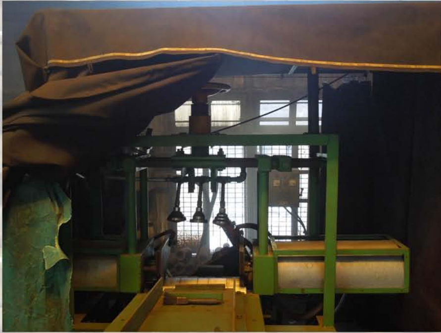
Magnetic Crack Detection ( wet method ) for finished springs
