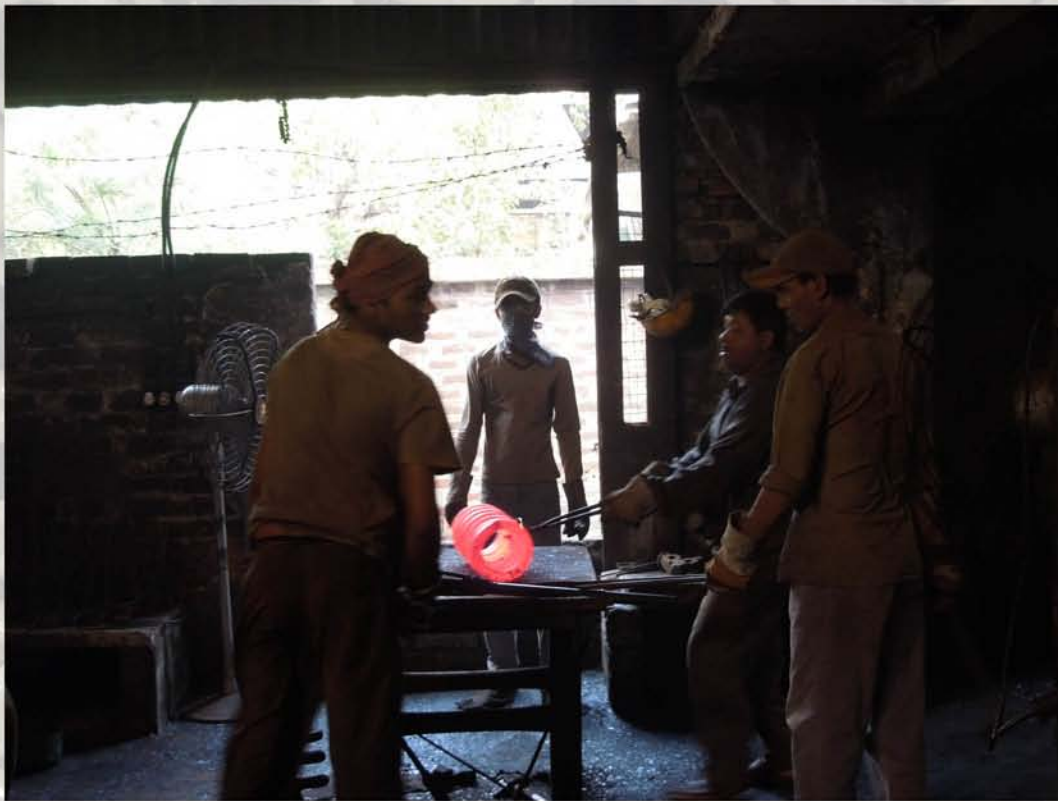
Sealing of open ends after coiling
