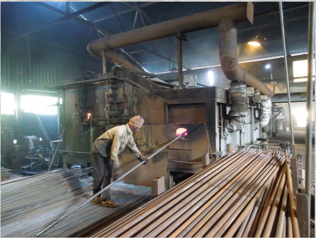
Worker inserting steel rods for coiling into a First-In-First-Out Walking Beam Furnace
