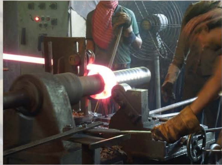
Coiling of heated bars into Helical Springs
