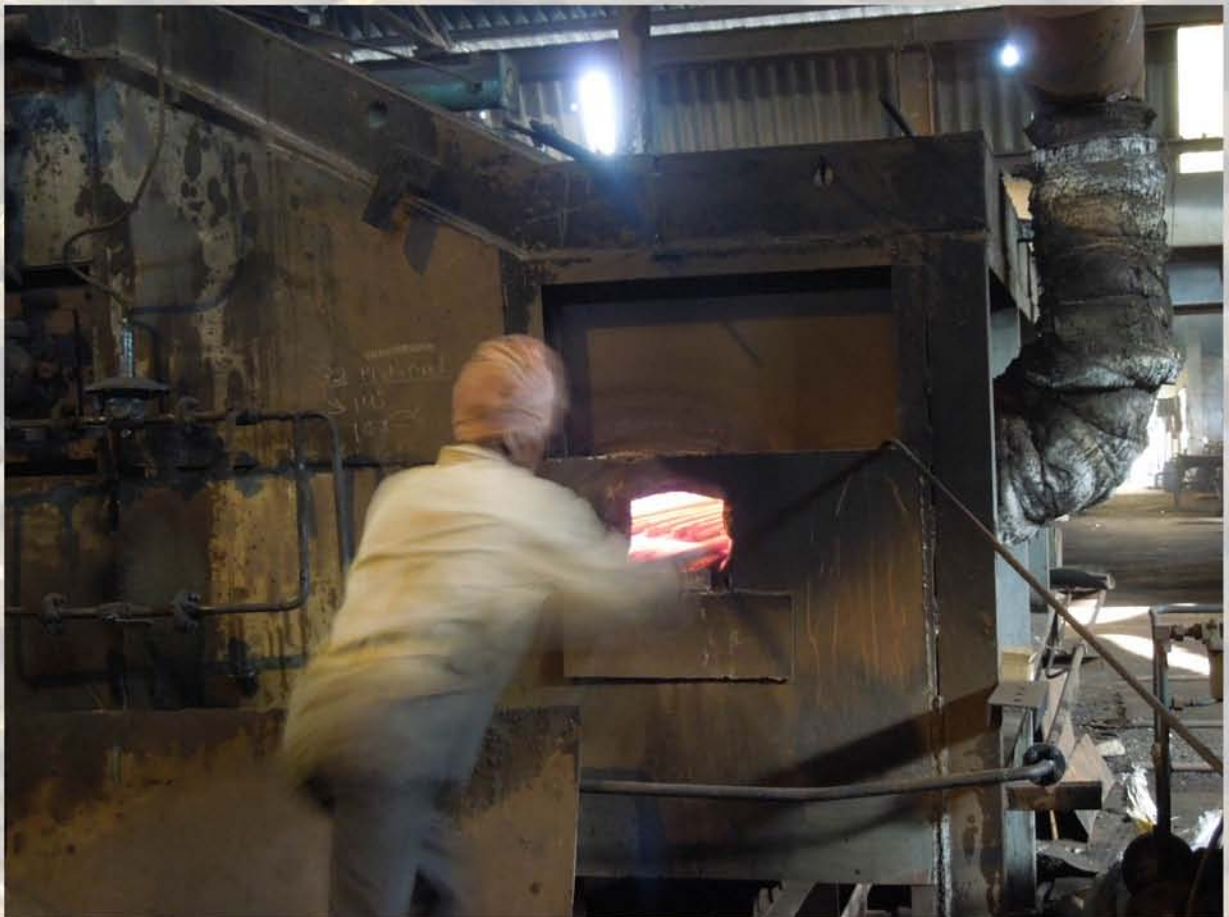
Worker inserting steel rods for coiling into a First-In-First-Out Walking Beam Furnace
